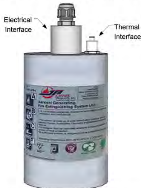
Figure 3 "Cylindrical type, Condensed aerosol fire extinguishing unit - activation interfaces"
