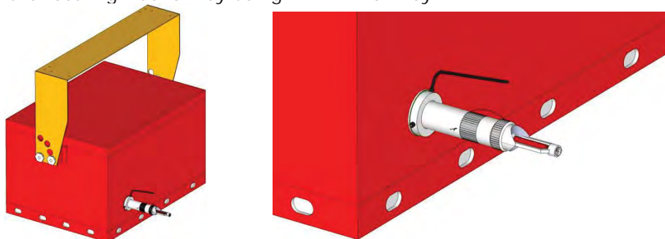
Figure 15 "Sealing the Bulb Thermal Actuator to the condensed aerosol fire extinguishing unit"
