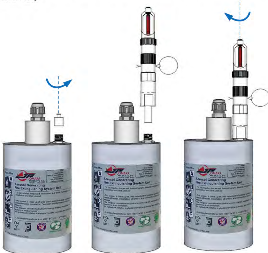
Figure 5 "Interfacing the Bulb Thermal Actuator to the condensed aerosol fire extinguishing unit"
